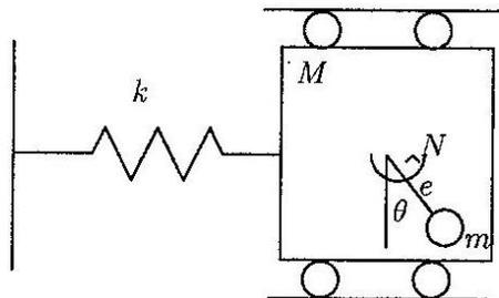
With  $y = x_3$  as the output, determine the relative degree and the zero dynamics. Give a physical interpretation of the zero dynamics.
