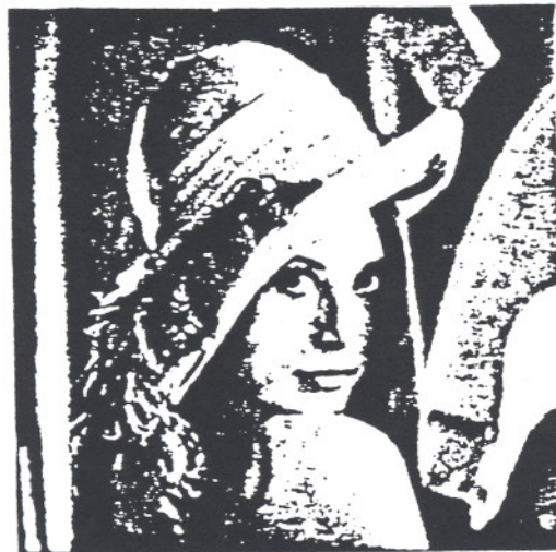
Figure 10.28 DM-coded image at 2 bits/pixel. The original image used is the image in Figure 10.22(a). NMSE = 2.4%, SNR = 16.2 dB.
