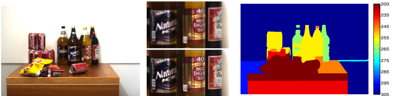
Figure 1: Left: Image captured using our coded aperture. Center: Top, closeup of captured image. Bottom, closeup of recovered sharp image. Right: Recovered depth map with color indicating depth from camera (cm) (in this this case, without user intervention).
