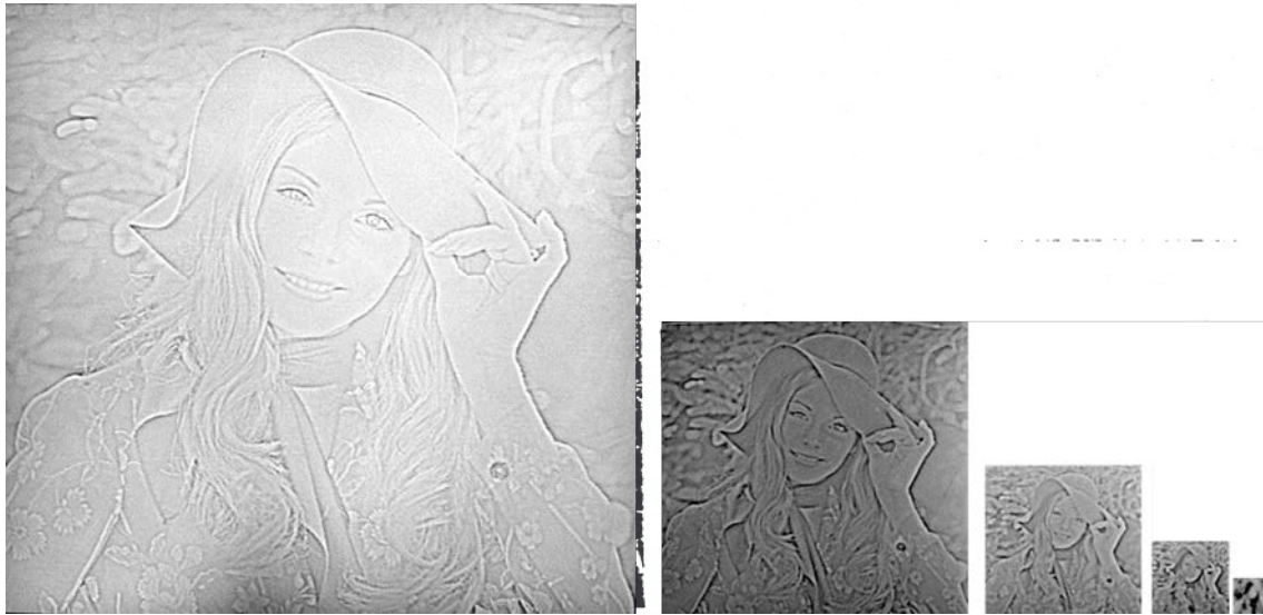
Figure 10.38 Example of the Laplacian pyramid image representation with K = 4 . The original image used is the 513 \times 513 -pixel image f_0(n_1, n_2) in Figure 10.36. e_i(n_1, n_2) for 0 \leq i \leq 3 and f_4(n_1, n_2) .
