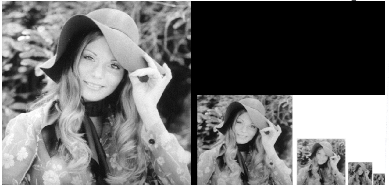
Figure 10.36 Example of the Gaussian pyramid representation for image of 513 x 513 pixels with K=4 .
