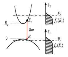
and the refractive index of the semiconductor is 3.5. In calculating  $f_C$  and  $f_V$ , you can assume charge neutrality, i.e., electron concentration is equal to hole concentration, and assume the doping concentration is negligible compared with injected electrons/holes.
