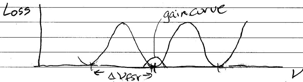
A very useful narrowband filter element is the Fabry-Pérot Etalon [read Svelto 4.5]
