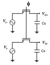
$$\begin{split} V_{o+} - V_{o-} &= V_{od} \quad V_{i+} - V_{i-} = V_{id} \\ V_{oc} &= \frac{V_{o+} + V_{o-}}{2} \quad V_{ic} = \frac{V_{i+} + V_{i-}}{2} \\ V_{o+} &= V_{i+} (I + \varepsilon_I) + V_{os1} \\ V_{o-} &= V_{i-} (I + \varepsilon_2) + V_{os2} \\ V_{od} &= V_{id} + V_{id} \frac{(\varepsilon_I + \varepsilon_2)}{2} + (\varepsilon_I - \varepsilon_2) V_{ic} + V_{os1} - V_{os2} \end{split}$$
