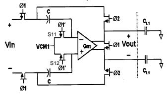
Offset voltage associated with charge injection of S11 & S12 cancelled by differential nature of the circuit
