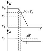
$$\begin{split} &C_{ov}=0.1fF/\mu \quad C_{ox}=9fF/\mu^2 \quad V_{th}=0.4V \quad V_L=0 \quad V_t\\ &\varepsilon=-\frac{C_{ov}}{C_s}=-\frac{10\mu x 0.1fF/\mu}{1pF}=-.1\%\\ &Allowing \ \varepsilon=1/2LSB \rightarrow ADC\ resolution <\sim 9bit \end{split}$$
