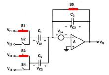
Sample mode (S1, S3, S5  $\rightarrow$  on S2, S4  $\rightarrow$  off)  $V_{C1}=V_{os}-V_{I1}$  ,  $V_{C2}=V_{os}-V_{I3}$ ,  $V_{C3}=0$   $V_{o}=V_{os}$
