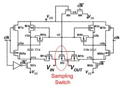
Ref: M. Waltari et al., "A self-calibrated pipeline ADC with 200MHz IFsampling frontend," ISSCC 2002, Dig. Tech. Papers, pp. 314
