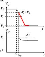
where  $\varepsilon = -\frac{C_{ov}}{C_s}$ ;  $V_{os} = -\frac{C_{ov}}{C_s} (V_{th} - V_L)$
