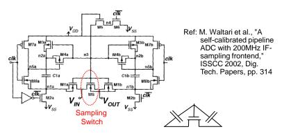
Two floating voltages sources generated and connected to Gate and S & D
