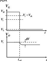
Sudden gate voltage drop → no gate voltage to establish current in channel
