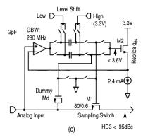
Ref: H. Pan et al., "A 3.3-V 12-b 50-MS/s A/D converter in 0.6um CMOS with over 80-dB SFDR," *IEEE J. Solid-State Circuits*, pp. 1769-1780, Dec. 2000
