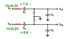
Track mode ( $\phi$  high)  $V_{C1}=V_{I1}$  ,  $V_{C2}=V_{I2}$   $V_{o1}=V_{o2}=0$
