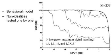
Effect of 1<sup>st</sup> Integrator maximum signal handling capability on converter SNR
