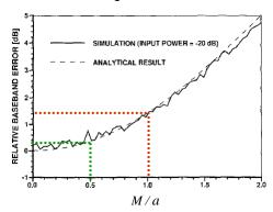
• Example:  $a = 2M \rightarrow 0.4$ dB degradation in SNR  $a = M \rightarrow 1.4$ dB degradation in SNR
