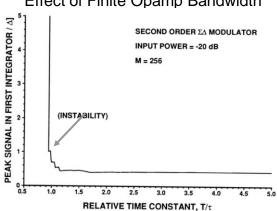
$ightarrow \Sigma \Delta$  does not require high opamp bandwidth  $T/\tau > 2$  or  $f_u > 2f_s$  adequate Note: Bandwidth requirements significantly more relaxed compared to Nyquist rate ADCs Ref: B.E. Boser et. al, "The Design of Sigma-Delta Modulation A/D Converters," JSSC, Dec. 1988.
