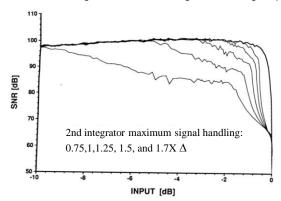
• Effect of 2nd Integrator maximum signal handling capability on SNR  $\rightarrow$  No SNR loss for max. sig. handling >1.7  $\Delta$
