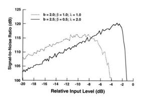
Effect of gain parameters on signal-to-noise ratio
