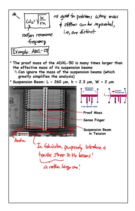
Tethers with fixed ends mass of stoucture >> mar of opmys : ignore the mass of springs Stiffness of springs << stiffness of the structure : ignore the stiffment of the structure For ADXL-50: 6070 of the mass comes from the some fingers -> M= 162 ng Suspension: Four tensioned becomes Guided B.C. Fixed B.C. F/4 Bending compliance k<sub>b</sub>-1 F/4 Stretching compliance  $k_{st}^{-1}$
