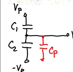
$$\begin{aligned} V_0 &= -V_p + (2V_p) \frac{C_1}{C_1 + C_2} \\ &= -V_p C_1 - V_p C_2 + 2V_p C_1 \\ &\Rightarrow V_0 = V_p \left( \frac{C_1 - C_2}{C_1 + C_2} \right) \quad (\text{ideal}) \end{aligned}$$
