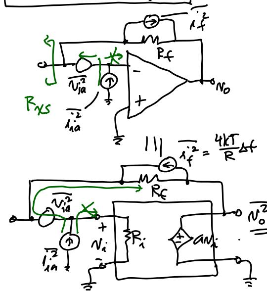
Get  $\overline{N_o^2}$ : use superposition  $\rightarrow$  handle one noise source at a time
