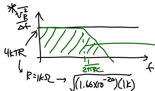
$$1k\Omega: 4nV/\sqrt{Hz} \quad (\text{for every } 1k \text{ of } R)$$
