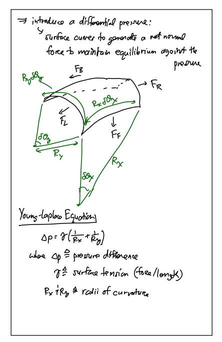
Contact Angle ] - governed by a balance of surface tensions usually proporty dependent on the interface between different marientals Example. Hydrophilic Droplet fea liquid-air surface torrion force fle - liquid-solid intenface fa = adherian force Solid-air synface tonsion force Equilibrium: 1) ho isomtal forces cancel and contact pt. fa: forsing fra=fos+flacosoc Tos+ Pros+ Procosoc [for of 87 ] Relationship between Surface tenrious captured by contact angle.
