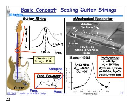
Brute Force Methods for Resonance Frequency Determination
