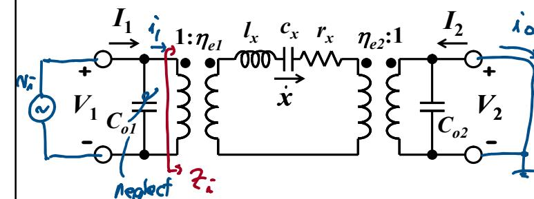
$$\dot{x} = \frac{1}{n_{e1}} i_1 \quad \dot{i}_o = \frac{n_{e2}}{n_{e1}} i_1 = \frac{n_{e2}}{n_{e1}} \left( \frac{N_i}{Z_i} \right) \quad (\text{neglecting } C_o)$$
