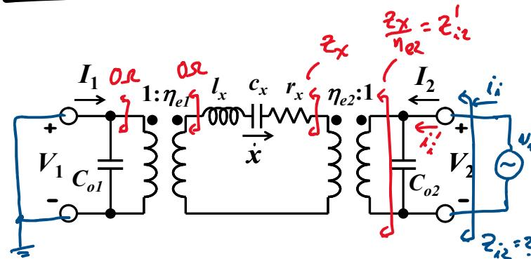
$$Z'_i2 = \frac{N_i}{i_i} \cdot \frac{Z_x}{n_e^2} = \frac{j\omega(l_x)}{n_e^2} + \frac{1}{j\omega(n_e^2 C_x)} + \frac{r_x}{R_{x2}}$$
