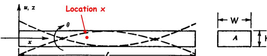
$$\text{Equivalent Mass} = M_{eq,x} = \frac{K.E.}{\frac{1}{2}V_x^2} = \frac{\frac{1}{2}\rho A \int_0^l V^2(x) dx}{\frac{1}{2}V_x^2}$$
