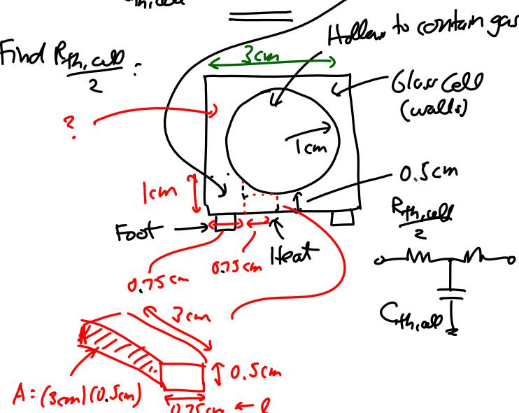
$$R_{th} = \frac{l}{KA} : R_{th,cell} = \frac{3}{2} \frac{1}{k(3)(\frac{1}{2})} + \frac{3}{k(3)(1)} = \frac{1}{k} \left( \frac{1}{2} + \frac{1}{1} \right) = \frac{3}{2k}$$
