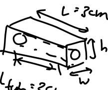
$$V_{cell} = hWL - \pi R_{tube}^2 \cdot L_{tube}$$
