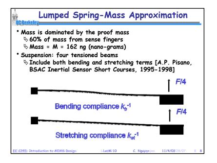
Suspension Beam in Tension
