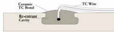
Fig. 1.2: In the 1501 structure, the thermocouple is mounted in the center of a re-entrant cavity, filled with alumina based cement (the bond area).
