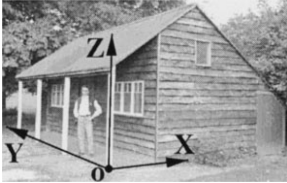
Figure 14. Computing the location of the camera: Equations (18) are used to obtain: X_c = -381.0 cm, Y_c = -653.7 cm, Z_c = 162.8 cm.
