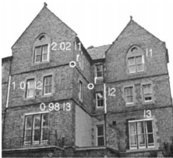
Figure 8. Measuring ratio of lengths of parallel line segments lying on two parallel scene planes: The points \mathbf{r} and \mathbf{r}' (together with the plane vanishing line and the vanishing point) define the homology between the two planes on the facade of the building.
