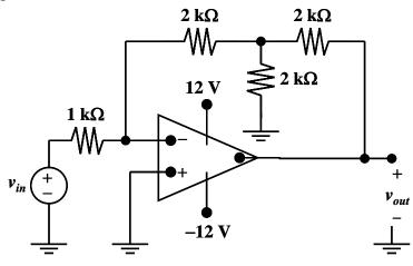
a) Assuming the op amp is operating in its linear region, find an expression for  $v_{out}$  (as a function of  $v_{in}$ ). [10 pts]
