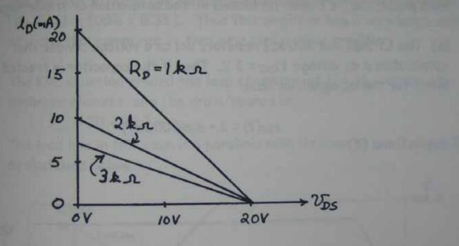
Notice that the load line rotates around the point ( $V_{DD}$ , 0) as the resistance changes.
