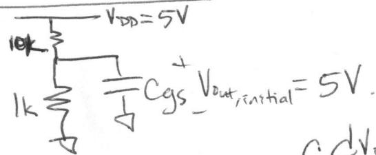
$$C \frac{dV_{out}}{dt} + \frac{V_{out}}{1k} = \frac{V_{DD} - V_{out}}{10k}$$
