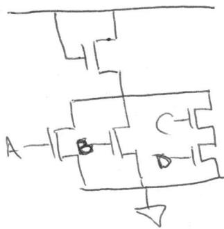
$$V_L = V_{DD} \left( \frac{R_{P, \text{on}, \text{largest}}}{R_{P, \text{on}} + R_{N, \text{on}, \text{largest}}} \right)$$
