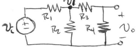
$$V_o = V_i \left( \frac{R_4}{R_3 + R_4} \right) \quad V_1 = V_i \left( \frac{R_2}{R_1 + R_2} \right)$$
