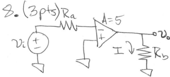
Summing point constraint cannot be applied for this problem because  $A \ll \infty$  and there is no negative feedback
