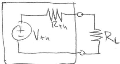
$$P_L = \frac{V_L^2}{R_L} = \frac{V_{th}^2 \left( \frac{R_L}{R_{th}+R_L} \right)^2}{R_L} = \boxed{\frac{V_{th}^2 R_L}{R_{th}^2 + 2R_{th}R_L + R_L^2}}$$
