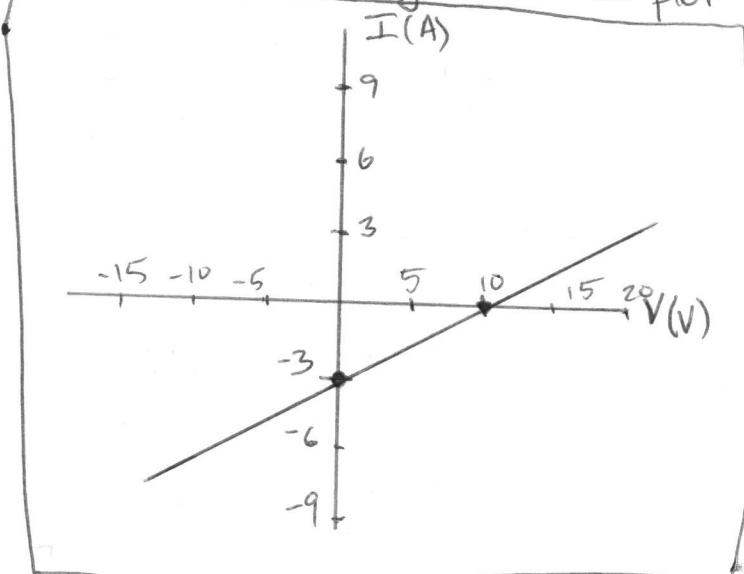
OR With the two points we can use the point-slope formula  $(V_1, I_1) = (10, 0)$ ,  $(V_0, I_0) = (0, -3)$
