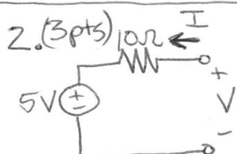
Since both elements are linear, their I-V characteristics will also be linear. If we can find two points on the I-V curve we are done.
