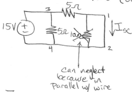
$$I_{sc} = \frac{V_3 - 0}{5\Omega} = \frac{15}{5} = 3A$$
