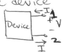
Find  $V$  when  $I=0$  (output is open circuit).
