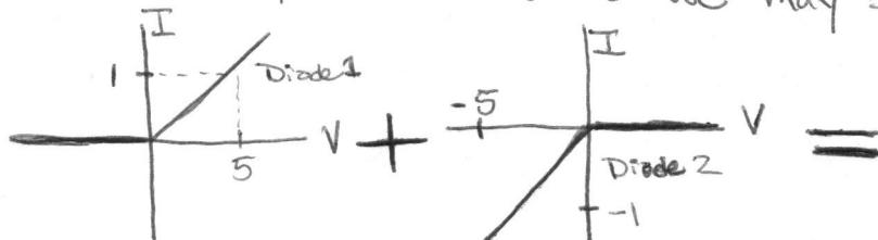
Note that  $I$  and  $V$  are the applied current / voltage in the circuit, not the passive reference direction current/voltage for the element.
