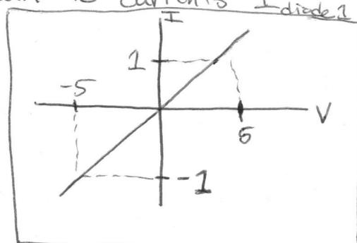
This is the I-V characteristic of a  $5\Omega$  resistor!
