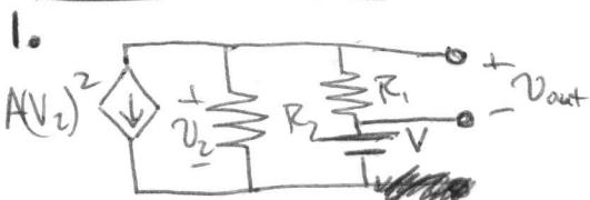
No, this circuit does not have a Thévenin equivalent. The concept of Thévenin or Norton equivalent circuits only applies for networks consisting of only linear elements. Since the dependent source is nonlinear, we cannot find a Thévenin (or Norton) equivalent.
