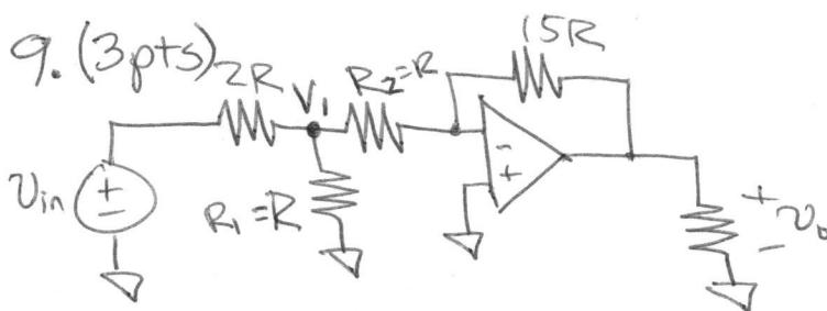
Have negative fb so summing pt. constraint applies.  $V^+ = 0V \Rightarrow V^- = 0V$ . Need to find the current through  $R_2$ .
