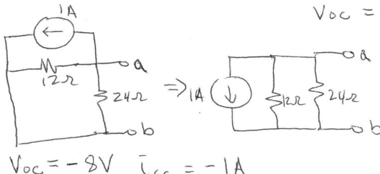
$$V_{oc,\text{tot}} = -16V$$
