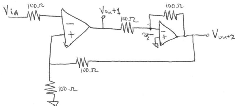
a.  $V_{out2} = -A(V_2^-) \Rightarrow V_2^- = -\frac{V_{out2}}{A}$  {  $V_1^+ = V_{out2}(\frac{1}{2})$
