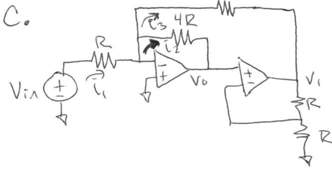
$$V_1 = \frac{V_o}{2} \quad (\text{basic non-inverting topology})$$
