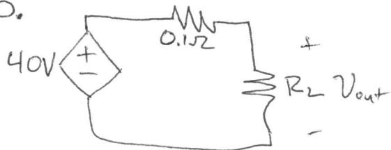
$$V_{out} = \left( \frac{R_L}{0.1 + R_L} \right) \cancel{40}$$
