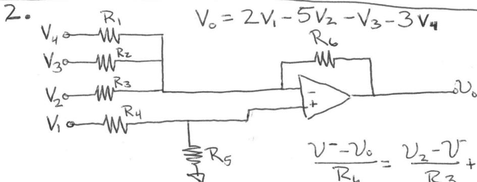
$$V^+ = V_1 \left( \frac{R_5}{R_4 + R_5} \right) = V^-$$
