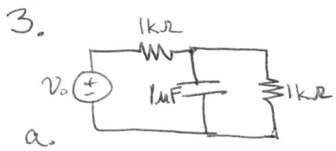
$$v_0 v_c(t) = \frac{1}{1k\Omega} \left( C \frac{dv_c(t)}{dt} + \frac{v_c(t)}{1k\Omega} \right)$$
