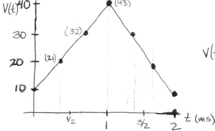
$$v(t) = \int_0^t \frac{i(t)}{C} dt + V_0$$
