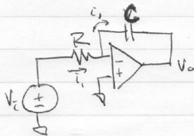
a. By summing pt const.  $i_1 = \frac{V_i}{R}$ ,  $V_o = -\frac{1}{j\omega C} i_1 = \frac{V_i}{j\omega RC}$
