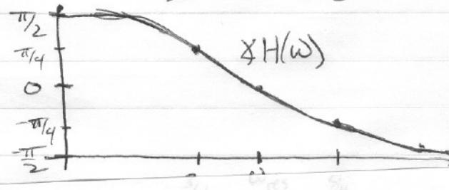
c.  $L = 1H, C = 1mF, R = 2\Omega, \omega_{res} = \frac{1}{\sqrt{LC}} = 1k \frac{\text{rad}}{\text{sec}}$
