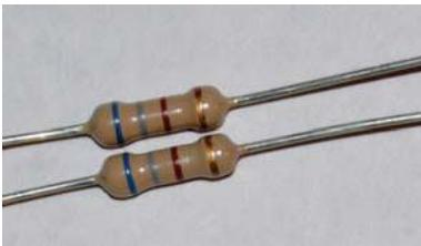
**Figure 1** A resistor with value  $680\ \Omega$  and 5 % tolerance (colors blue-grey-brown-gold).
