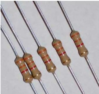
**Figure 2** Color coded resistors (colors orange-orange-red-gold).
