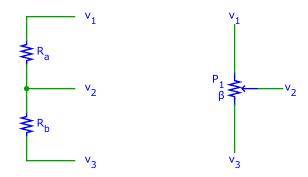
**Figure 3** Potentiometer: Equivalent circuit diagram (left) and symbol (right).
