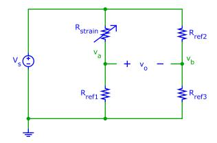
Figure 2 Full bridge configuration.
