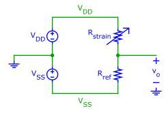
**Figure 1** Strain gage in a half bridge circuit configuration.
