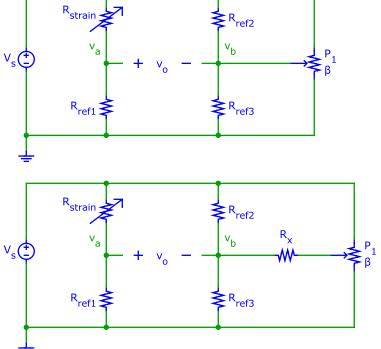
**Figure 4** Full bridge circuit with potentiometer for offset adjustment.
