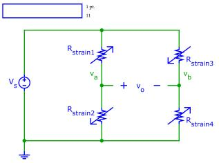
**Figure 6** Balanced full bridge circuit with four strain resistors.
