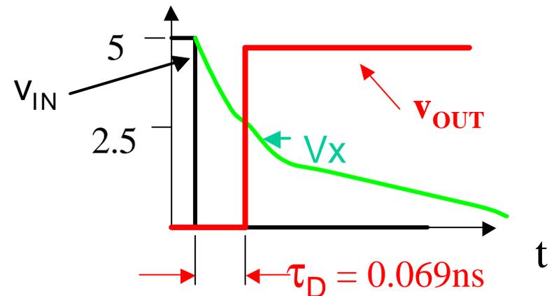
$RC = 0.1\text{ns}$  so  $0.069\text{ns}$  after  $v_{IN}$  switches by 5V,  $V_X$  moves 2.5V
