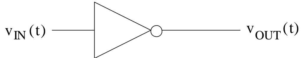
The delay is mostly simply the charging of the capacitors at internal nodes.
