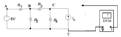
Thus we can connect the + lead of the DVM to point (Node) A and call the potential of point A  ${}^{\text{\tiny t}}V_{A}{}^{\text{\tiny t}}$ , similarly at points (Nodes) B, C.
