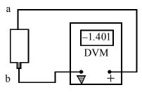
With this circuit, you are measuring  $V_a$  with respect to  $V_b$  (or  $V_a$  -  $V_b$ ). DVM indicates -1.4, so  $V_a < V_b$  by 1.4 V. Which is the positive battery terminal?
