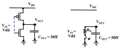
$$\Delta t = 0.69 R_D C_{OUT} = 0.69 (10 k\Omega) (50 fF) = 345 ps$$
