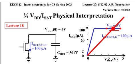
$\ensuremath{^{3}\!\!/_{4}}\ V_{DD}$  is the average value of  $\ensuremath{\,V_{OUT}}$
