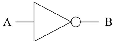
Using the result from the truth table above, draw how you will construct a NOT gate using a NAND gate.
