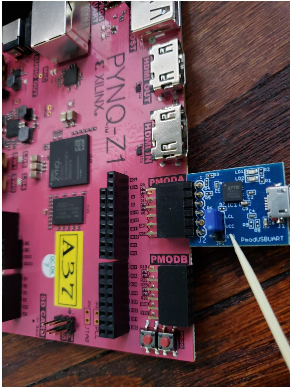
Figure 3: Pmod USBUART plugged in w/ correct power jumper setting (blue).
