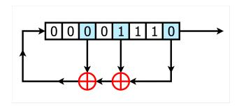
On each rising edge of the clock, you will shift the contents of the register 1 bit to the right. On the left side, you will shift in a single bit equal to the Exclusive Or (XOR) of the bits originally in position 0, 3, and 5. Note that in the diagram, the leftmost bit is bit 7 and the rightmost bit is bit 0.
