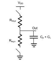
(a) Say  $R_{eq,n} = R_{eq,p} = 5m\Omega$  and  $C_P = C_{in} = 2nF$ . What is the propagation delay of an inverter in this design? [2 pts]
