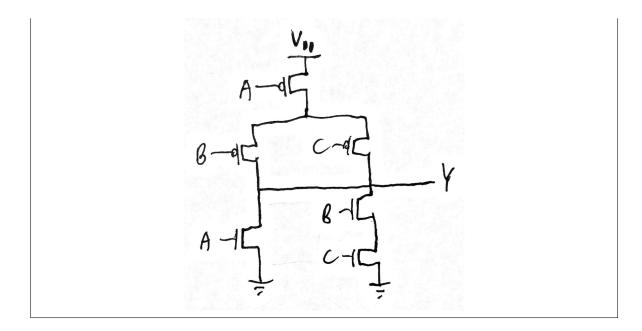
(d) Implement the logic function  $Y = \overline{A(B+C) + \overline{B}C}$  using a complementary pull-up and pulldown network. For this question, assume you have  $\overline{A}$ ,  $\overline{B}$ , and  $\overline{C}$  available in addition to A, B, and C. [2 pts]
