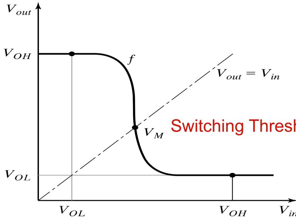
$$\begin{aligned}V_{OH} &= f(V_{OL}) \\V_{OL} &= f(V_{OH}) \\V_M &= f(V_M)\end{aligned}$$
