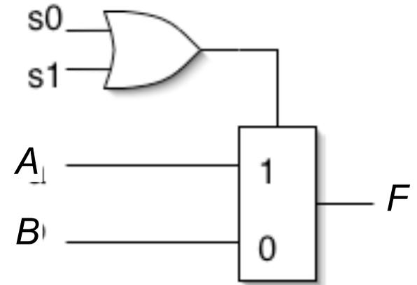
Should expand if-else into 4-bit wide multiplexor and optimize the control logic and ultimately to 4 4-LUT on an FPGA:
