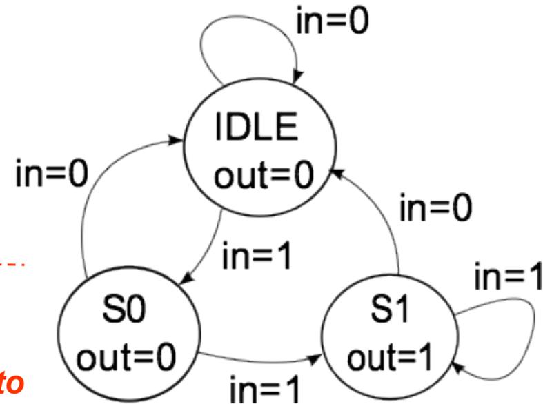
**A separate always block should be used for combination logic part of FSM. Next state and output generation. (Always blocks in a design work in parallel.)**
