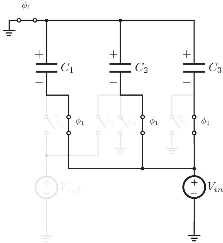
$$Q_{C_{1,2}} = (V_1 - V_{ref})C_1$$
