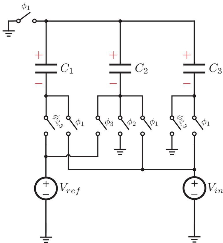
Note that all the capacitors are charged to the same voltage, i.e.  $-V_{in}$ , in this phase. You might astutely observe that they are in parallel. If you did *not* astutely observe this, fear not. You don't need to have done so to solve this circuit.
