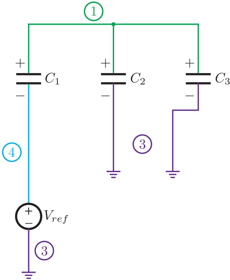
Yes, it's node 1. Give yourself a pat on the back! This means that the poor charges had nowhere to go between *all three phases*. All they've been able to do is haplessly scurry from plate to plate, perhaps searching for escape from the weird green maze but finding none.
