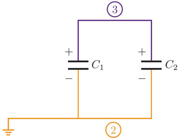
determined by charge that exists from the previous phase. To find this voltage, we continue with our procedure. Write the charge on each capacitor.
