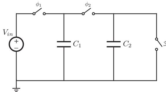
The switches labeled  $\phi_1$  are closed in phase 1 and open in phase 2. The switches labeled  $\phi_2$  are open in phase 1 and closed in phase 2. When a
