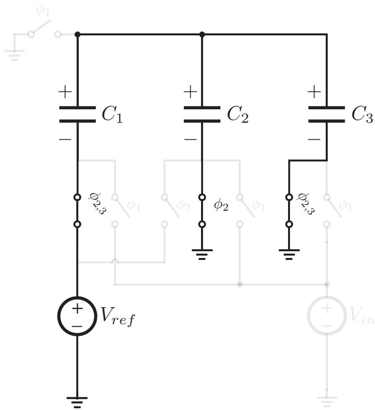
is part of the circuit. By the way, if you don't want to be identifying weirdly colored pieces of metal that charges are going to be trapped in, i.e. if electrons aren't your thing, worry not. There's an easier way to identify floating nodes. Any node that is not connected to a voltage source, current source or ground is going to be a floating node. Simply because there will be no source or sink of charge connected to that node.)
