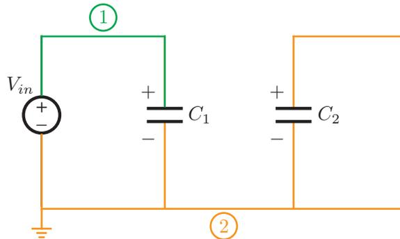
Now we continue with our procedure. All of the node voltages in this phase are known.  $V_1 = V_{in}$  and  $V_2 = 0$  is our reference voltage. We can use this to find the charge on each capacitor. Charge is given by capacitance  $\times (V_{+plate} - V_{-plate})$
