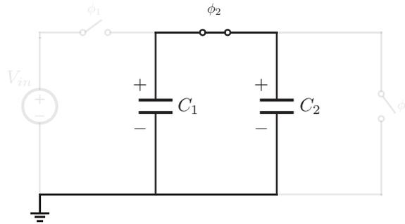
the circuit are greyed out so that you can see exactly how we modify the circuit between the two phases.
