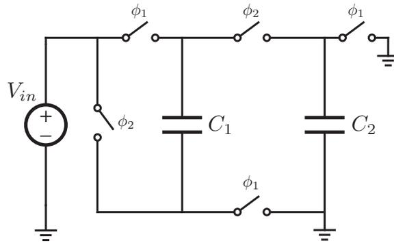
The switches labeled  $\phi_1$  are closed in phase 1 and open in phase 2. The switches labeled  $\phi_2$  are open in phase 1 and closed in phase 2. Begin the procedure:
