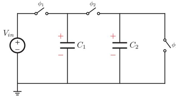
The reason that we write these signs is to be consistent with charge polarity from phase to phase. You can think of it like a guess. We are guessing that the top plates of  $C_1$  and  $C_2$  have positive charges, and that the bottom plates have negative charges. It turns out that this guess does not matter. If this is confusing, try to flip the signs (- signs on the two top plates and + signs on the bottom plates) and go through the procedure. The result will be the same!
