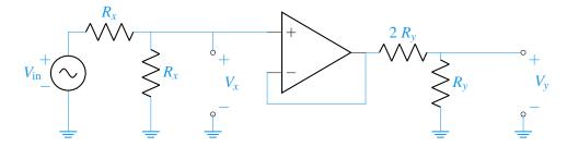
Since no current flow into the positive op-amp input, we've successfully isolated the dividers so they can be used in a modular fashion!  $\Box$
