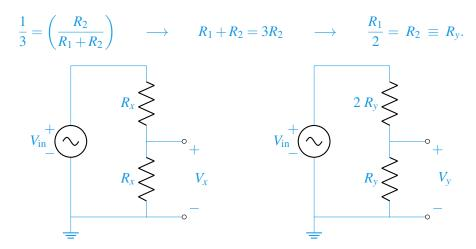
(b) If you combine the voltage dividers, made in part (a), as shown by the block diagram (output of the 1/2 voltage divider becomes the source for the 1/3 voltage divider circuit), do they behave as we hope (meaning  $6V_{in} = 3V_x = V_y$ )?
