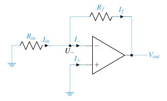
Note that  $R_f$  and  $R_{in}$  now form a voltage divider.
