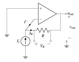
Calculate  $v_{\text{out}}$  as a function of  $I_s$  and R.
