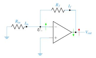
We suppose that the  $v_{out}$  goes up.  $v_{out}$  is connected to  $U_-$  so  $U_-$  also goes up. Our op-amp equation is  $v_{out} = A(v_+ - v_-)$ , so  $U_-$  going up will cause  $v_{out}$  to go down. This is the opposite of what initially happened, so we are in negative feedback.
