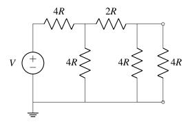
Answer: We want to find the equivalent resistance across the voltage source in Figure 6.2. Start by reducing the two resistors on the right to  $4R \parallel 4R = 2R$ . Then combine the other 2*R* resistor with this to get a new resistor of value 4*R* as in the circuit below.
