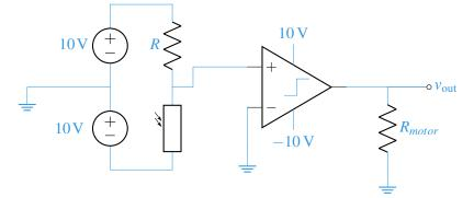
Since we have grounded the negative input terminal (and there is no feedback in the circuit), we realize the comparator rails high (positive  $v_{out} = +10V$  when the input to the positive op-amp terminal has positive voltage.
