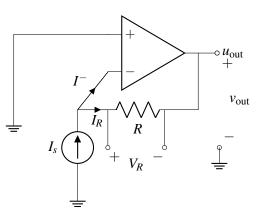
Calculate  $v_{out}$  as a function of  $I_s$  and R.
