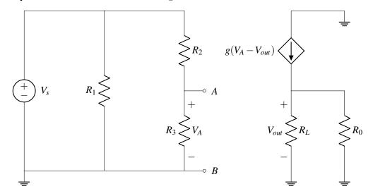
Find a symbolic expression for  $V_{out}$  as a function of  $V_s$ . Hint: Redraw the left part of the circuit using with its Thévenin equivalent.
