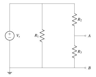
(b) Now a load resistor,  $R_L = R$ , is connected across terminals A and B as shown in the circuit below. Find the power dissipated in the load resistor in terms of given variables.
