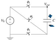
(a) In the circuit above switches  $\phi_1$  are initially closed and switch  $\phi_2$  is initially open. Calculate the value of the output voltage,  $V_{out}$  with respect to ground, and the amount of charge stored on capacitor,  $C$ , at that state (phase 1).
