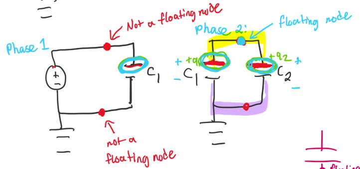
Floating node: charge doesn't flow in/out of the node
