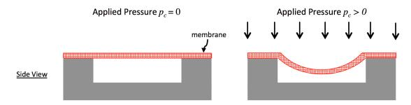
(a) You attach a resistor layer  $R_p$  with resistivity  $\rho = 0.1\Omega m$ , width W, length L, and thickness t to the pressure sensor membrane, as illustrated in the figure below. When the pressure  $p_c = 0$  Pa (i.e. there is no applied pressure), W = 1 mm,  $L = L_0 = 1$  cm,  $t = 100 \,\mu m = 100 \times 10^{-6}$  m.
