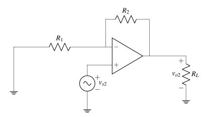
(c) Use the Golden Rules to find the output voltage  $v_o$  for the circuit shown below.
