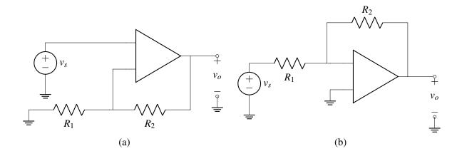
(a) Label the input terminals of the op-amp with (+) and (-) signs in Figure (a), so that it is in negative feedback. Then derive the voltage gain  $(G = \frac{v_o}{v_s})$  of the non-inverting amplifier in Figure (a) using the Golden Rules. Why do you think this circuit is called a non-inverting amplifier?
