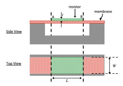
(b) When pressure is applied, the length of the resistor L changes from  $L_0$  and is a function of applied pressure  $p_c$ , and is given by
