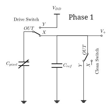
2. Disconnect clean switch from ground to enable charge storing
