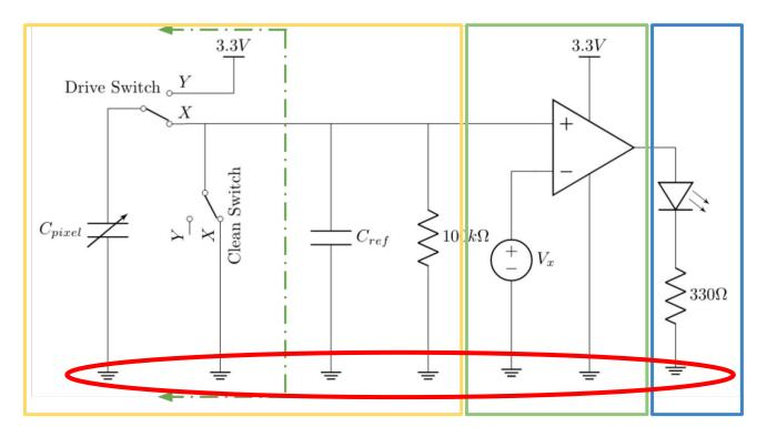
Note: these are all the same node! They are all connected to the breadboard ground rail.
