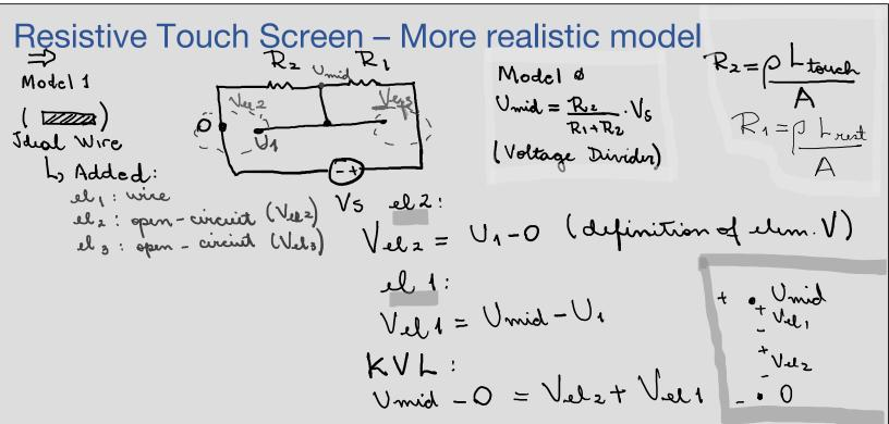
Resistive Touch Screen - More realistic model R2 Unid K1 Vela = U1-0 (definition of elem. V) Model 1 ( 122022) Ideal Wire Vell = Umid-U, Lo Added: els: open-circuit (Verz) els: open-circuit (Verz) KVL: Vmid -0 = Velet Vell Un= Velz Umid -U1 = Vel1 J Umid = Vel1 + Velz Umid -U1 = Vel1 J Umid = Vel1 + Velz O= pleV: svin a in 1 le Umid = 0 + Velz = Velz = V1 \* By measuring Val 2 ve get Unid for any Ltouch.
