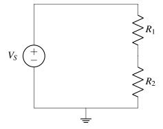
• Step 2: Label the node connected to the voltage supply as  $u_1 (= V_S)$ , since the voltage supply goes between this node and ground.
