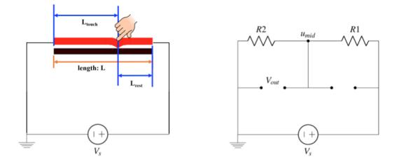
Does the voltage at  $u_{mid}$  change in this case? Thinking about it in terms of nodal analysis, we have not actually added any new nodes to our circuit - ideal wires (with zero voltage drop) are all that we have actually added. Therefore, we see that with a perfect conductor (analogous to our ideal wire),  $V_{out} = u_{mid}$ .
