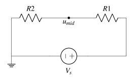
To understand what the bottom plate is doing, we will first assume the bottom plate is a perfect conductor  $(\rho = 0)$ , so the circuit will look as follows. Notice again that a voltage source is connected to the terminating edges of the top plate:
