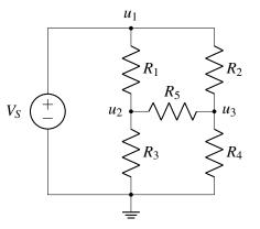
• Step 2: Write equations for the nodes with voltage sources between them. Here, the ground node and  $u_1$  have  $V_s$  between them, which tells us that
