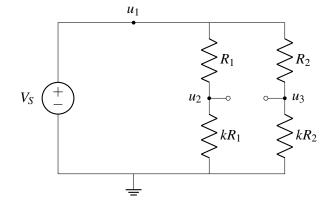
Now, we can write  $u_2, u_3$  directly, using the voltage divider equation as we did above:
